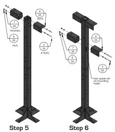
Assemble arms to upper column as shown. Tighten all fasteners to 10 ft-lbs.
