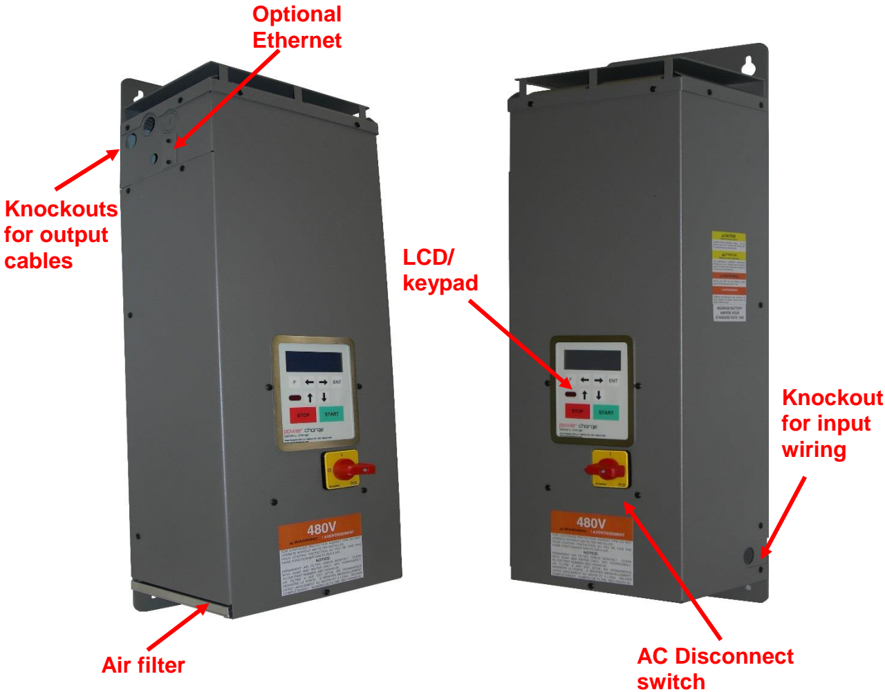
Figure 1: PowerCharge™ iHF3 6 kW Battery Charger features
