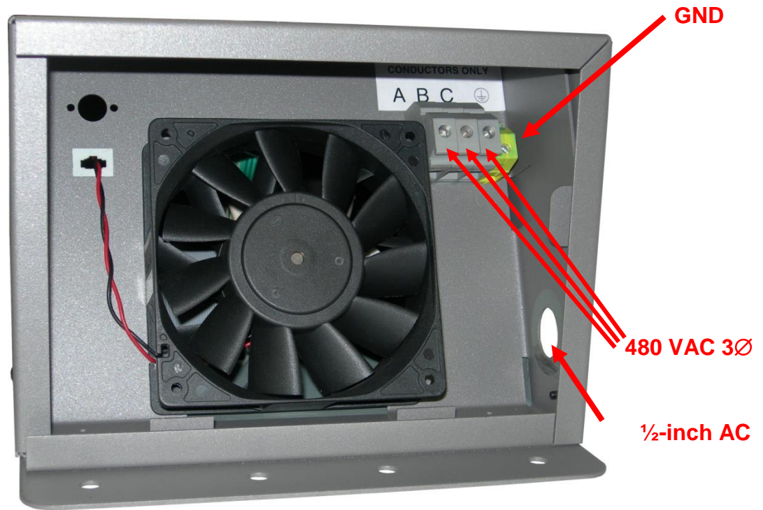
Figure 11: Charger electrical connection points
